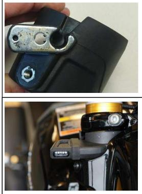
Install the new indicators onto the rubber brackets.
