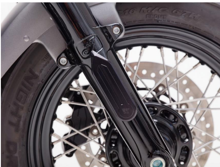
Cover to hide the reflectors
