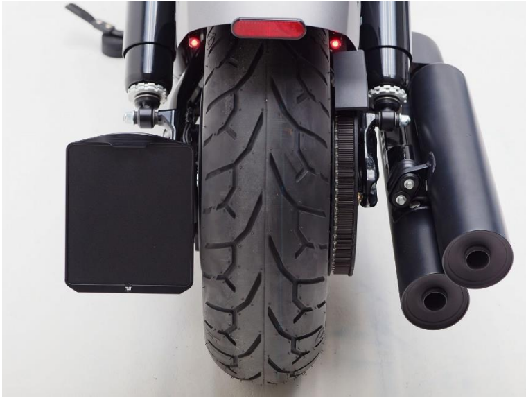
Side license plate holder and lighting
