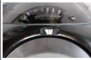
Remove the protective film from the windshield. Using the screws and washers provided, attach the windshield to the mask.
