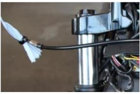
Drain the brake fluid according to the manufacturer's specifications and loosen the brake line from the brake pump.
