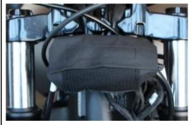
Put the cables and their plug connectors back into the protective cover.
