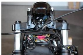
Remove the handlebar switches from the handlebar.
