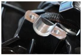
Insert the reduction into the top yoke.
