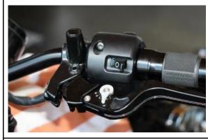
Unclip the clutch cable.
