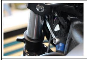
Align the fairing and attach it using a fork wrench.
