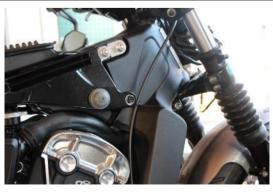
Attach the cable to the frame using a cable tie
