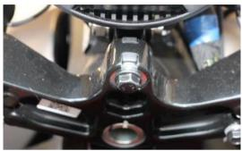
Attach the headlight to the lower top yoke using the original screw.
