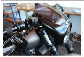
Slide the fairing onto the headlight and into the brackets. In doing so, the two brackets of the mask must be inserted between the spacer washers and the washers.
