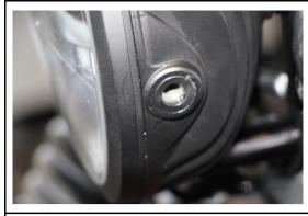
Insert the spacer washers into the headlight.
