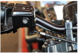
Replace the original brake lines with the ones provided.
