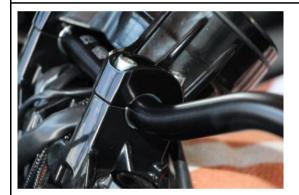
Insert the handlebar (type 0330) into the top yoke, align and attach.
