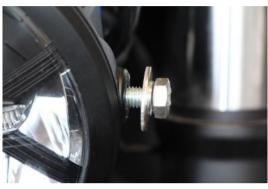
Screw in the screws, safety washers and washers into the headlight.
