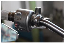
The final assembly of the operating elements requires the drilling of holes for the centring pins. To do this, align the operating elements and mark the positions for the centring pins (push onto the pins using grease).
