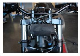
Run the clutch cable and the brake line in such a way that they do not touch the fairing when installing.
