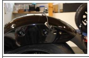
Remove the cable harness for the tail light from the holders.
