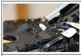
Disconnect the plug connector of the indicators.
