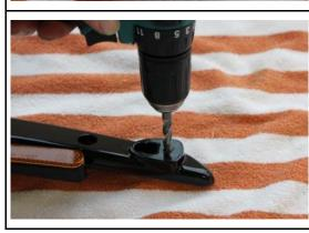
Drill out the fixing hole to 8mm.
