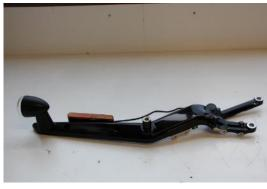
Completely remove the left rear bracket of the fender.
