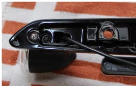
Unscrew the indicator from the bracket and detach the cable from the holders.
