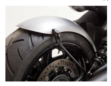
Rear fender conversion kit: seat, mudguard, struts incl. LEDs
