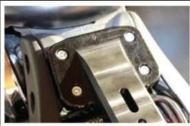
Insert the rubber cover of the holder into the notch as well.
