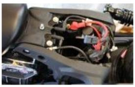
Remove seat. Disconnect the battery, unclip holder and electrics and remove the battery.
