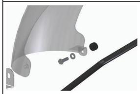
...attach to the swingarm using the screw (M6), a washer and one of the spacer sleeve provided (check for central position of the fender) as well as the original brake line holder. Only lightly tighten screw at this moment.
