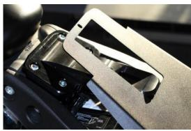
Cover the rear fender and carefully slide the battery cover over the holder.
