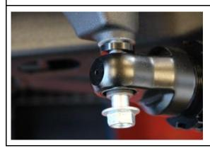
First, loosen the upper screw of the shock absorber on the left and insert a provided spacer between the shock absorber and the frame. The original washer is omitted. **Caution: When loosening the screw, the spring strut should be neither under pressure nor under tension.** Reattach the shock absorber.
