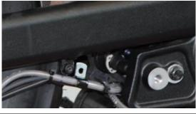
Loosen the holder for the brake line on the right side of the swingarm.
