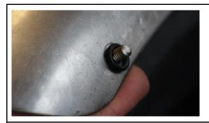
Attach the braces with the screws, washers and o-rings...
