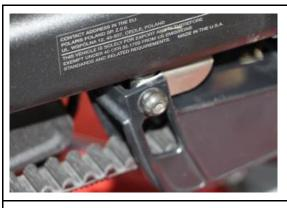
Mount the belt guard with the holder using the original screws.
