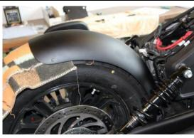
Carefully slide the fender into the swingarm and ...
