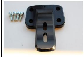
Screw the seat holder onto the original tank holder using the screws and safety washers provided.
