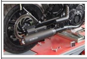
Remove the upper silencer and cover the lower silencer with a cloth.
