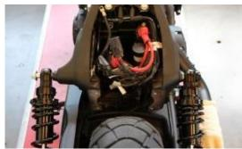
Disconnect the plug for the rear lighting.
