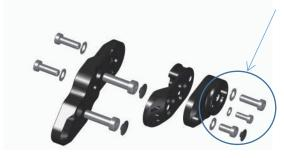
Attach the footrest mounting to the adjusting plate using the screws and safety washers provided.
