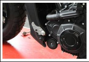
Loosen both fastening screws of the original footrest and remove the complete unit.
