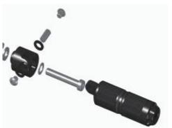
Attach the footrest with the threaded bush, the plastic washers (moisten with grease) and both screws (M8).
