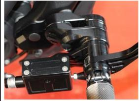
Attach the brake cylinder onto the bracket.
