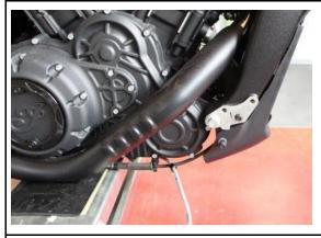
Loosen both fastening screws of the original footrest and remove the complete unit.
