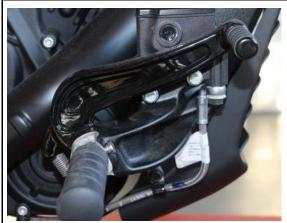
Cover manifold and exhaust with a cloth or towel. Remove the bracket of the brake line.
