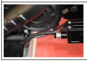
Attach the brake line with the banjo bolt provided using new seals to the brake cylinder as shown.
