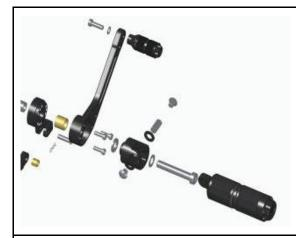
Bigger changes can be achieved with the removal of the lever and its twist to the reversing lever. During the subsequent installation, note the following tightening torques:
