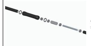
Counter the threaded rod and socket with the nut and slide on the cover.
