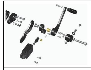
Screw the joint mount with brake lever, reversing lever (with bearing) and brake cylinder bracket onto the footrest mounting as shown.
