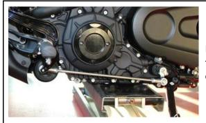
Remove the original shift linkage. Unscrew the two nuts from the original shift linkage and screw them onto the one provided.
