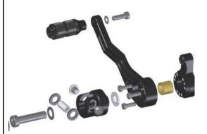
Bigger changes to the lever position can be achieved with the removal of the lever and its twist to the reversing lever. During the subsequent installation, note the following tightening torques:
