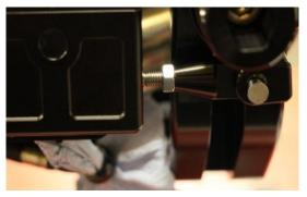
By screwing in and unscrewing the push rod, the position of the foot brake lever can be adjusted exactly. Then counter the push rod with the nut.
