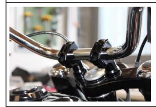
Insert the handlebar into the risers, align and attach lightly.
