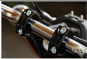
Align the handlebar as desired and tighten.
