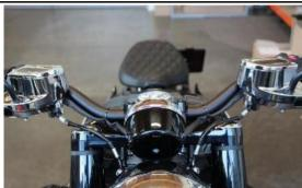
After the final assembly, check the freedom of movement of the brakelines and wires and fasten them only to such an extent that they are not bent, do not chafe and are tension-free in maximum steering angle and over the entire spring travel.
