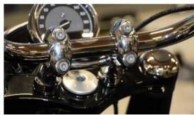
Loosen the two screws of the original risers under the top yoke by approx. 5 rotations.
