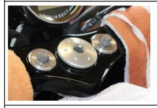
Fully loosen both screws under the top yoke.
