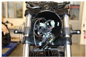
Disconnect the plugs of the indicators in the head-lamp housing.
