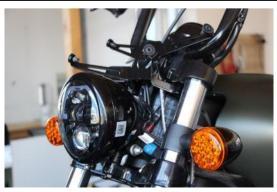
Loosen all retaining screws on the front mask and remove it.
