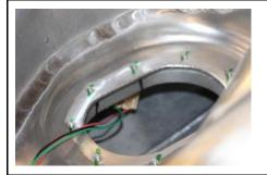
Remove the pump halfway and unplug the cable from the floater. Then remove the fuel pump completely.
