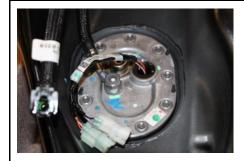
Loosen all screws of the fuel pump.
