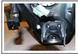
Remove the original holder and attach it to the aluminium tank.
