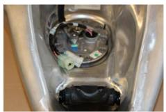
Mount the floater and fuel pump into the aluminium tank as per the original.
