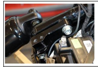
Attach the two connection brackets to the frame on both sides using the original screws.
