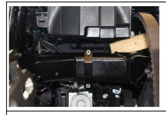
Mount the fender holder provided on the swingarm in such a way that...
