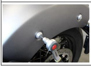
Unscrew and remove the rear fender.
