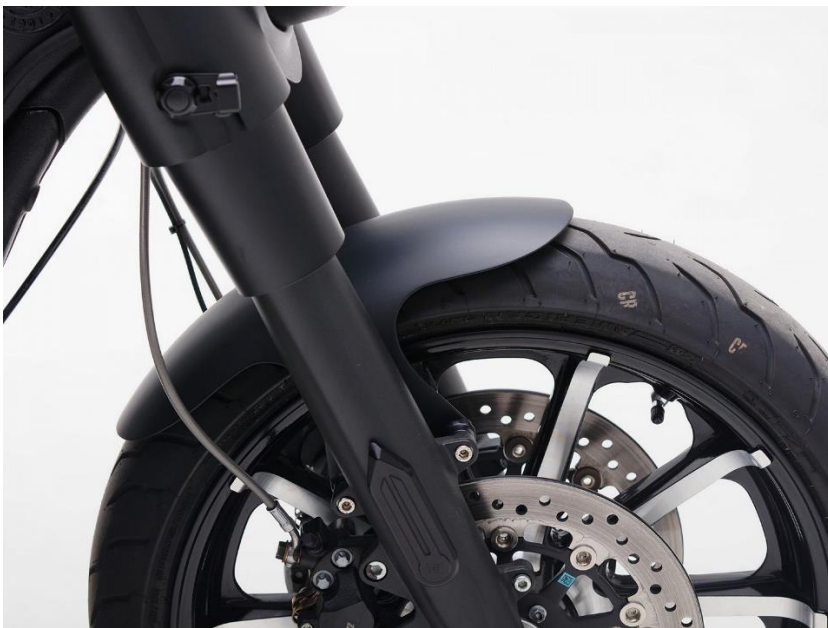
Shortened front fender & Covers for the side reflectors
