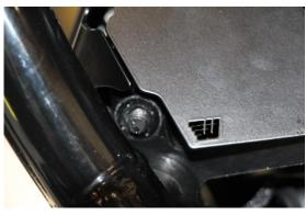
Mount the cover to the holder of the horn on the left side. To do this, place the screw and washer provided through the holder from the inside. Screw onto the original nut.
