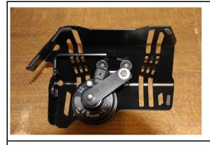
Attach it to the horn using the spacer bushing, screw, washer and nut provided (alignment see image) to the cover.
