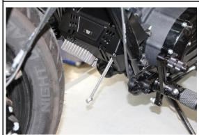
Align the cover and tighten the screw.
