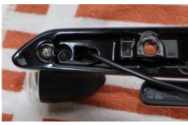
Unscrew the indicator from the rear support and detach the cable from the adhesive holders.
