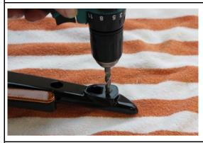
Drill out the fixing hole to 8 mm.
