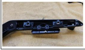
Attach the cable to the bracket with the holders.
