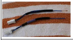
Cut the connectors of the original lighting and solder them to the cable ends according to the plan using the supplied solder connectors. Observe the polarity.
