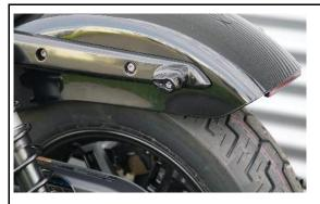
Mount the rear bracket to the vehicle. Fix all removed parts on the left side.
