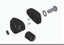
Attach the enclosed tail light/indicator combinations to the bracket with an adapter, safety washer and screw.
