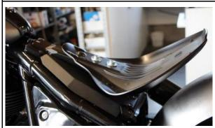
Attach the seat shell onto the holder using the screws and large diameter washers provided, adjust as required and tighten.
