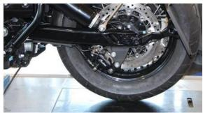
Lay both rear light cables along the swingarm so that they can be connected to the battery.
