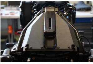
Place the holding frame onto the connection brackets and the vehicle frame and compare the positions of the holes with the corresponding threads.
