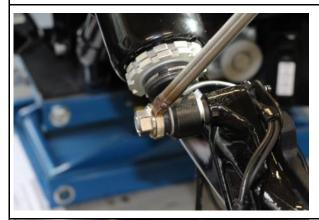
Mount the two supporting braces for the rear fender to the lower fixing points of the spring struts using the nuts provided.
