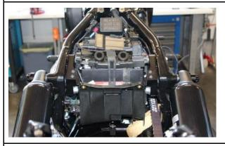
Reattach the battery using the original bracket. Place the complete electrics in front of the battery box and attach.
