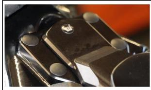
Push the plastic coverings into the screw heads and stick in the pin.
