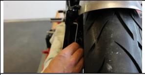
Another setting option exists by the thread pins on the inside of the rear lights.
