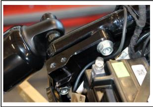
Attach the two connection brackets to the frame on both sides using the original screws.
