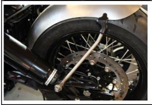
Attach the fender to the struts at the rear using the screws, washers and rubber rings.
