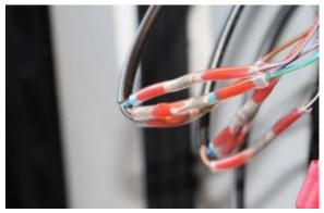
Connect the cable harness provided with the rear lights and the original plug using the solder connectors according to the diagram.
