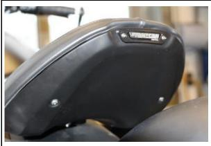
Attach the emblem using the two screws (M4) provided.
